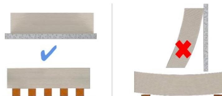
If the boards are subsequently moved around the site, they should be placed on a level surface with sufficient support for lifting by forklift. store boards undercover and keep dry prior to fixing. if the boards become wet allow drying before fixing is commenced. in any case, boards should be installed in position within 2-3 weeks of procurement.
